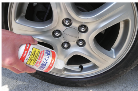
STEG 1: Injicera EMERGENCY TYRE SEALANT i däck
